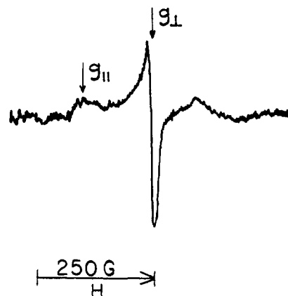
Figure 3. ESR spectrum of O_2^- formed in the photolysis of oxygen-saturated 0.02 M formate solution at pH 11.7, g_{\perp} = 2.006 , g_{\parallel} = 2.103 ; sample at 95 K.
